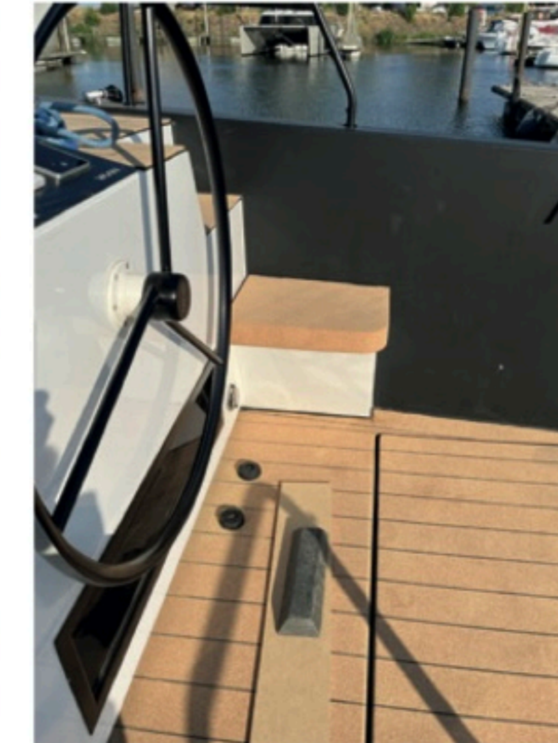
The steering wheels control the rudders via a Jefa linkage system. It's direct and gives a good feeling of control at the helm. You can also steer sitting on the step.
