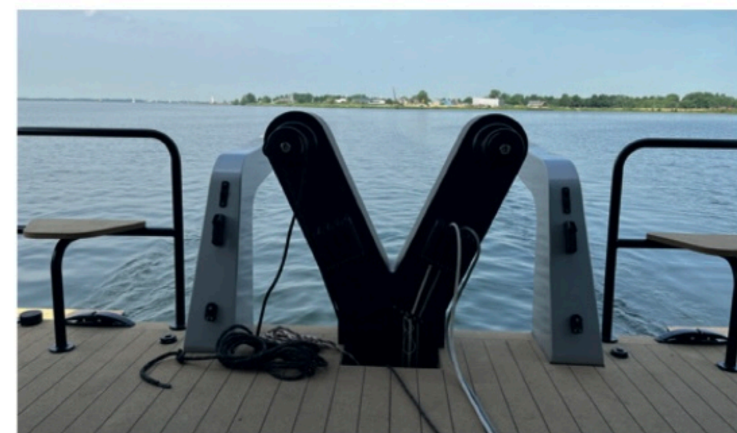
The central V-shaped post displays the brand's logo. All halyards, the mainsheet and jib sheets are led to electric winches that can be controlled from the helm stations.
