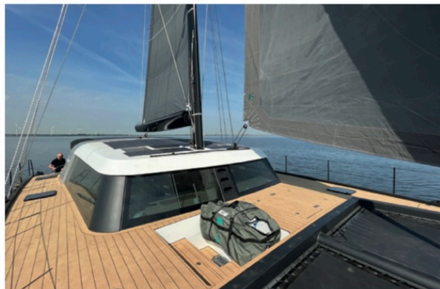
The cork deck is extremely comfortable underfoot and contrasts elegantly with the black of the hull. As a material, it offers excellent insulation as well as being a truly ecological product. Note the integrated steps for easy access to the coachroof - they too will be lined with cork.
