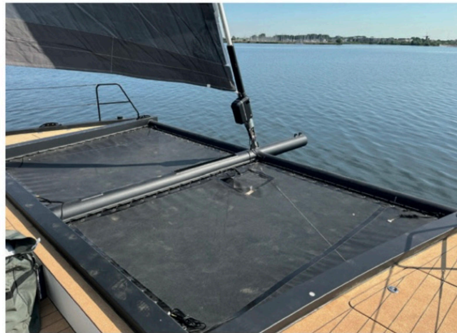
The forward beam cross-setup may seem a little rustic with its round aluminum tubes. Some might even see a touch of retro-elegance in it... Note that the rigidity of it means that an unsightly martingale is not required here.
